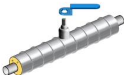
Air vent/drain units 5.6.1.
